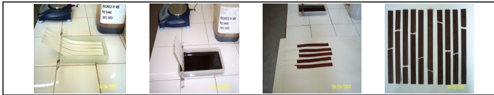
Fig. 3 – Testing of mechanical properties on the filter paper impregnated with adhesive lignocellulose systems
